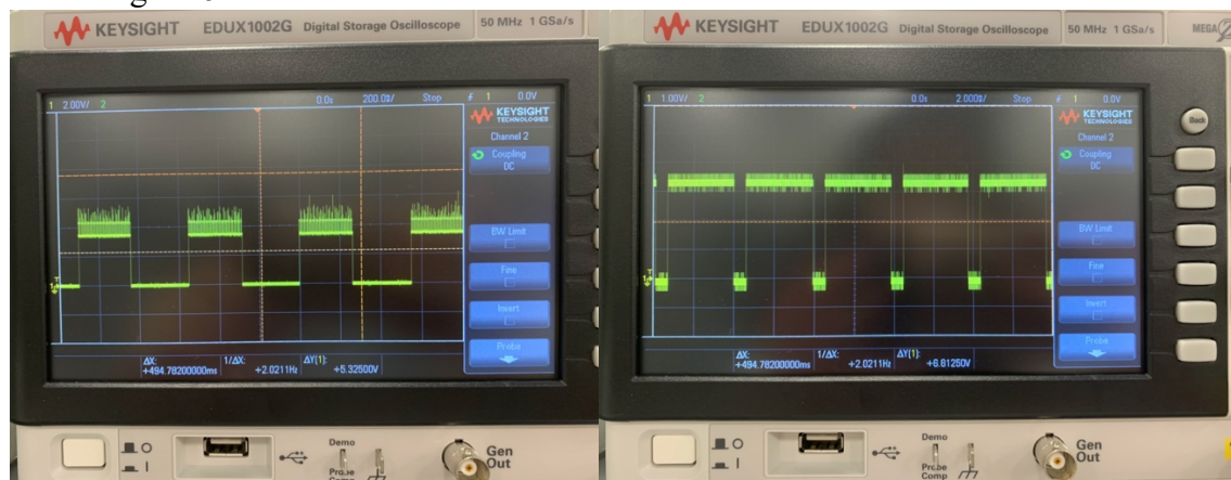
Figure 6b: Oscilloscope images of 2Hz 50% duty cycle blinking LED (left) and maximum brightness ~300Hz continuous LED (right)
